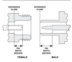
Before mating an unknown or new device with your 371XXA Port connectors or calibration devices, always measure the pin depth of the device's connectors. Use a ANRITSU Pin Depth Gauge, or equivalent, for these measurements (Figure C-2). Also, measure the connector pindepth of a device when intermittent or degraded performance is suspected.
