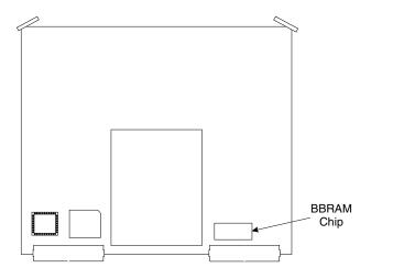
Figure 8-3. Location of BBRAM Chip on the A9 PCB
