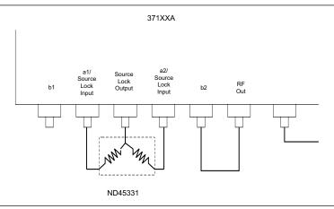
Figure 4-6. Noise Floor/Receiver Dynamic Range Setup
