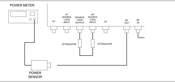
Figure 4-4. b2 Channel Verification Setup
