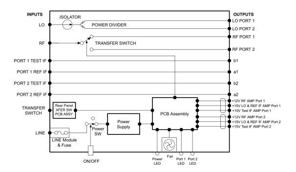
Figure E-4. 3735B Test Set Overall Block Diagram
