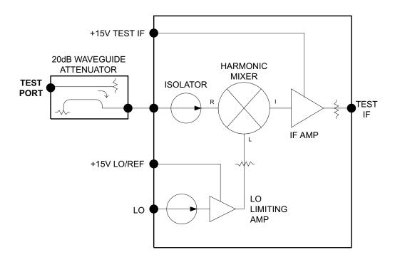
Figure E-7. 3741A-X Millimeter Wave Module Block Diagram
