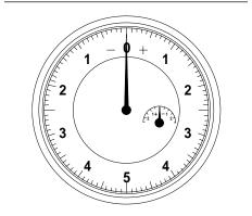
Figure C-2. Pin Depth Gauge
