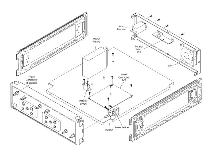
Figure E-8. Replaceable Parts Exploded View
