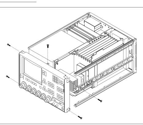
Figure 8-6. Removal of Front Panel Assembly
