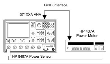
Figure 6-1. Equipment Set-Up for RF Power/ALC Calibration
