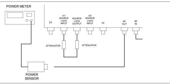
Figure 4-3. b1 Channel Verification Setup
