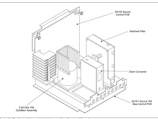
Figure 8-15. Signal Source Module Assemblies Removal Details
