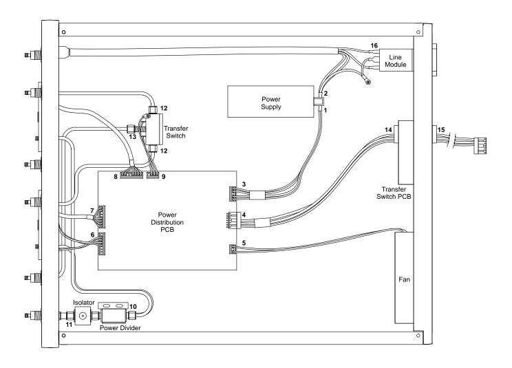
Figure E-9. Wiring and Connectors on Replaceable Part (Keyed to Removal Procedures)
