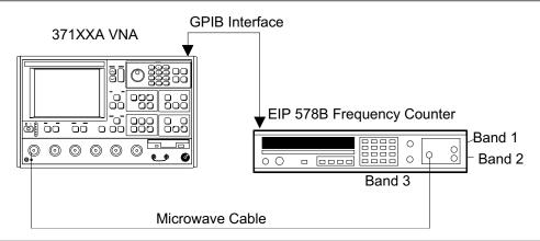
Figure 6-2. Equipment Set-Up for Frequency Calibration
