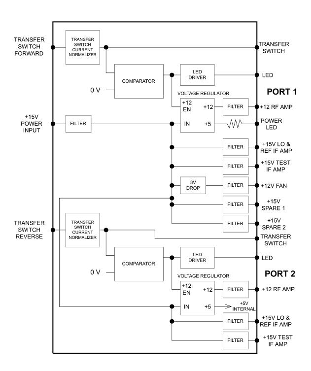
Figure E-5. 3735B Test Set PCB Assembly Block Diagram
