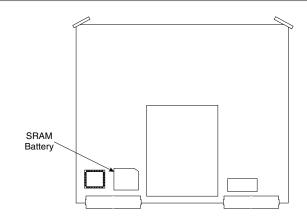
Figure 8-4. Location of SRAM Battery on the A9 PCB
