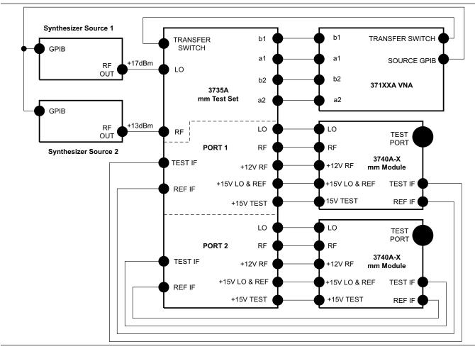
Figure E-3. 371XXA Millimeter Wave VNA System Interconnections
