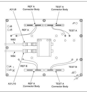
Figure 8-13. A31 Buffer Amplifier/Sampler Assembly, Details
