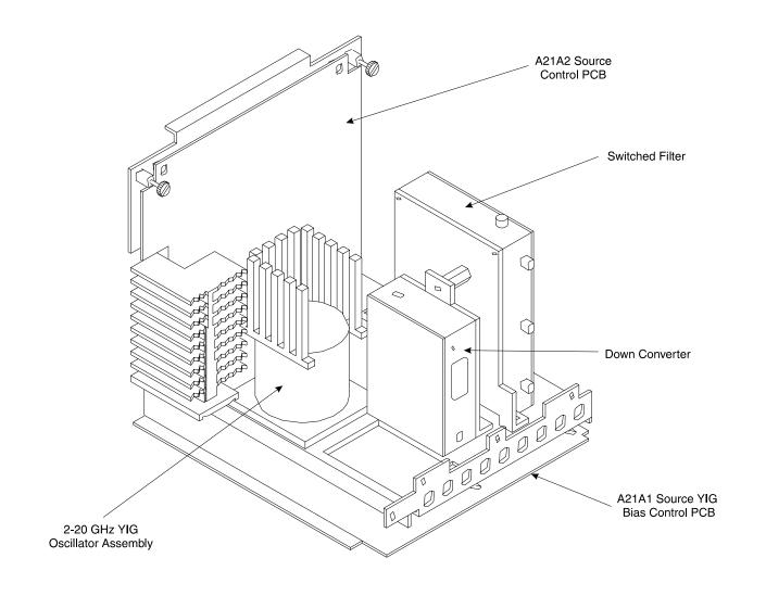
Figure 2-3. Signal Source Parts Location Diagram
