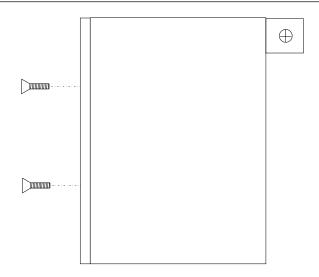
Figure 8-8. Location of Floppy Disk Drive Assembly Mounting Plate Screws
