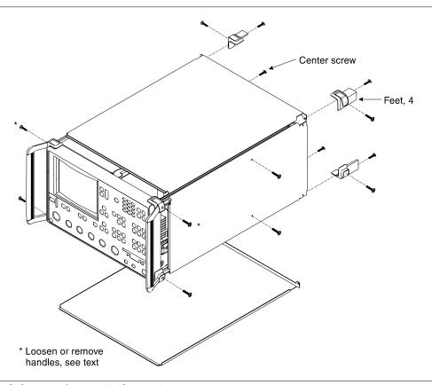
Figure 8-1. Exploded View of 371XXA Chassis Covers
