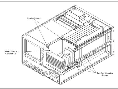
Figure 8-14. Signal Source Module Removal Details
