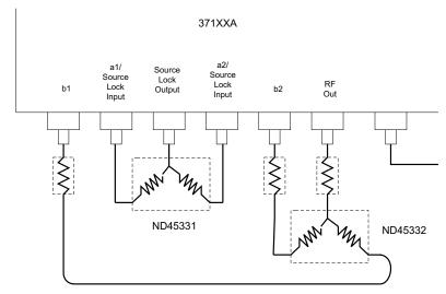
Figure 4-1. Connecting the Test Fixtures
