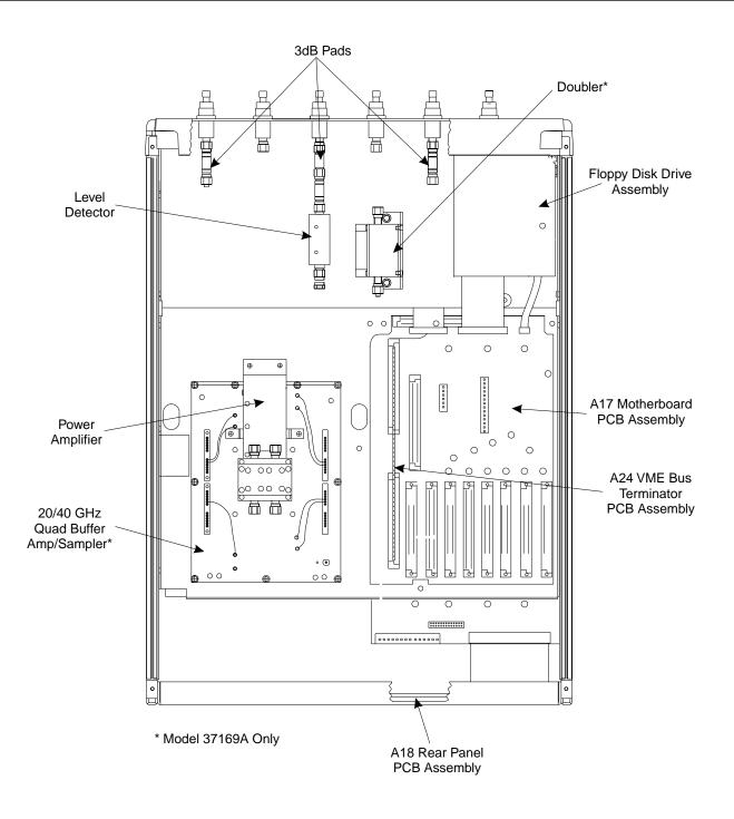
Figure 8-10. 371XX Module Components Layout Diagram
