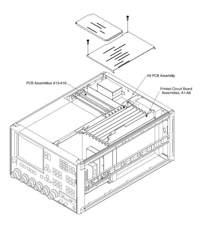
Figure 8-2. A1-A9 and A13-A16 PCB Assemblies Removal Diagram
