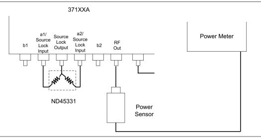
Figure 4-5. Source Power Level Setup
